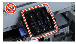
Use your fingers to turn the connector fixing screws (4 pc) counterclockwise to loosen them.
