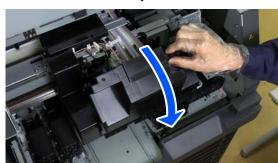
Turn all the fixing levers (4 locations) sideways to release the locks of the Ink Damper Unit.
