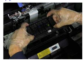
Place the used Print Head that you removed on the lid of the protective case.
